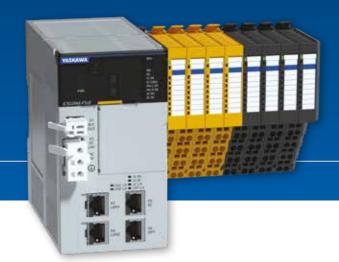
The iC9200 machine controllers are available with an integrated EtherCAT (FSoE) safety master, eliminating the need for an external safety PLC and allowing all safety and non-safety EtherCAT devices to be integrated onto a single network. Safety applications are programmed using certified safety function blocks in iCube Engineer, allowing you to use a single software engineering tool for programming safety and non-safety logic and motion.
